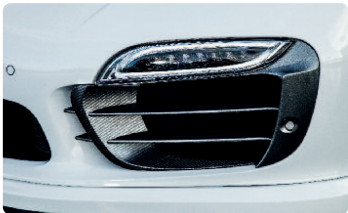
Aero Wings in Sichtcarbon, matt. Airblades in Titangrau Metallic lackiert. Aerowings in carbon fiber, matt finish. Airblades painted in Titanium Grey Metallic.
